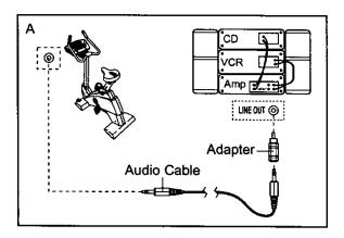
B. Plug one end of the audio cable into the jack beneath the console. Plug the other end of the cable into the adapter. Plug the adapter into an RCA Y-adapter (available at electronics stores). Next, remove the wire that is currently plugged into the LINE OUT jack on your stereo and plug the wire into the unused side of the Y-adapter. Plug the Y-adapter into the LINE OUT jack on your stereo.
